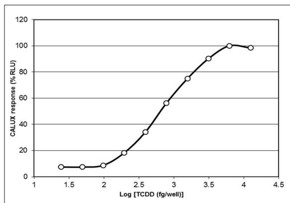
Figure 2. Example of a 10-point standard TCDD calibration curve
