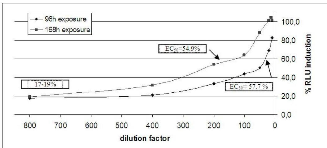
Figure 3. An overview of the dilution curves for two ceramic dosimeters with exposure times of 96 and 168 h
